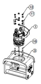
Place rotator (1) onto the swivel mount (3) and fasten with six bolts (10) and six locknuts (12) (torque to 150ft lbs).
