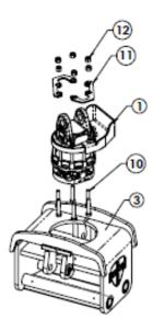
Place rotator (1) onto the swivel mount (3) and fasten with six bolts (10) and six locknuts (12) (torque to 150ft lbs).
